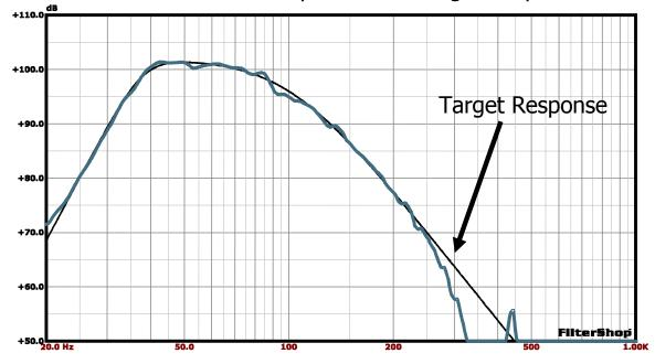
The Reference Target Response is an Acoustical Band-Pass Response of a total 10th order. High Pass=Butterworth 6th Order @ **38Hz**, Low-Pass=Linkwitz-Riley 4th Order @ **100Hz**
