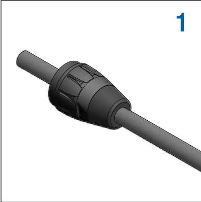
Slide the nut onto the cable
