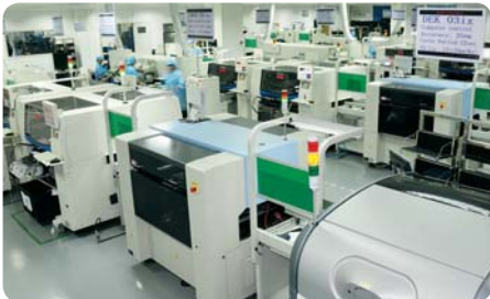
Cutting-edge Surface Mount Technology (SMT) makes fast and accurate work of loading circuit boards with miniaturized electronic components
