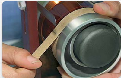
We wind over 100 different sizes of voice coils
