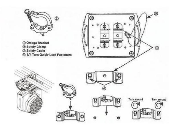
Regardless of the rigging option you choose for your 19pcs zoom, always be sure to secure your fixture with a safety cable. The fixture provides a built-in rigging point for a safety cable on the hanging bracket as illustrated above. Be sure to only use the designated rigging point for the safety cable and never secure a safety cable to a carrying handle.
