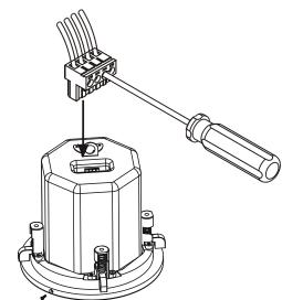
5.3 After the step1 and 2, put the unit into the ceiling round hole after inserting the input connector into the connecting socket of NCL-4/NCL-6.
