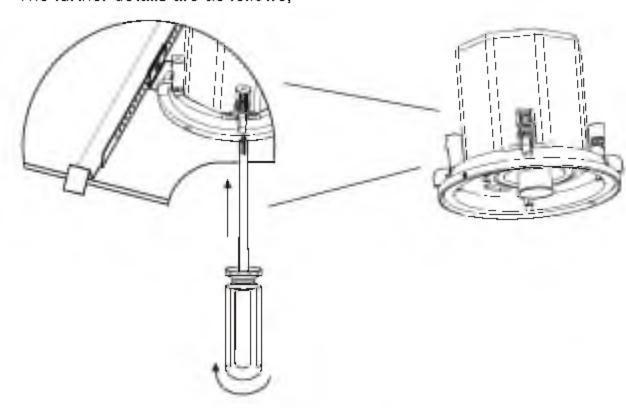
5.5 Then, you should select the required output power via the tap selector on panel. Finally, install the perforated press-in grille for ending the installation.
